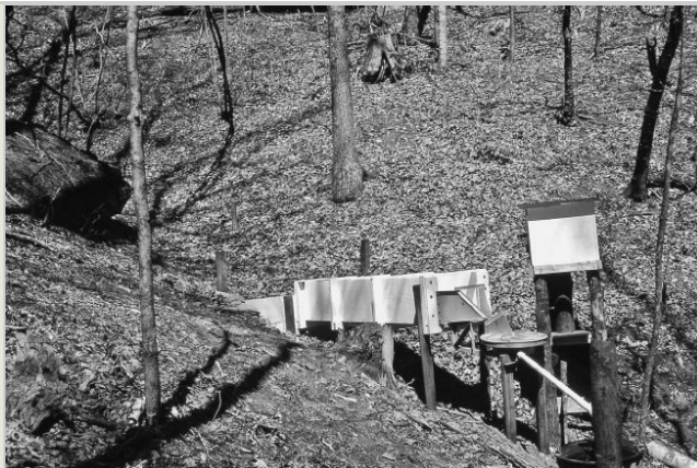
Figure 3.9 One foot H-Flume and Coshocton sampler (no. 701) on WS 7—one of four such installations used to assess water quality above and below roads, 1976.
