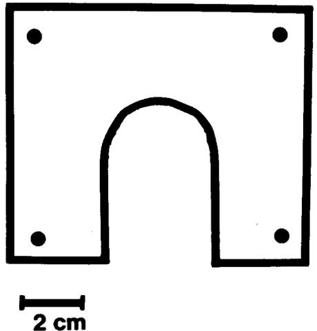
Fig. 1. Restrictor used to exclude other species and deter enlargement of red-cockaded woodpecker cavities in North Carolina.
